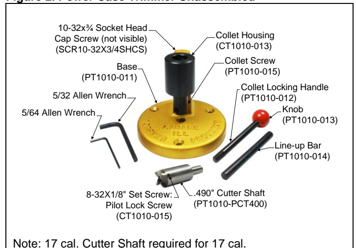
Figure 2. Power Case Trimmer Unassembled
