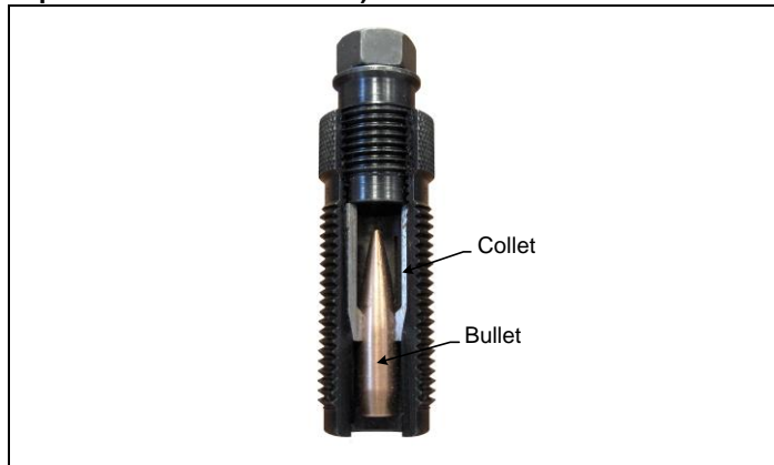
Figure 3. Cutaway of the Universal Bullet Puller (after bullet is pulled and before release)
