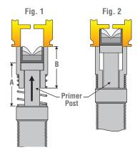
**Fig. 1** shows Dimension "A" greater than dimension "B" by .004" to .006". **Fig. 2** shows that when force is applied to the guide block of the press, the bottom of the primer cup stops against the base of the primer post. The top of the primer cup stops against the case head. Because the primer post is longer than the cup by .004" to .006", the primer will always be seated .004" to .006" below the case head.
