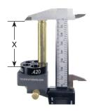
X = relative measurement between the base of a case to a datum point on its shoulder angle.
