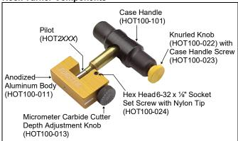
A standard case-holder handle is included, and a larger handle (HOT100-102) is required for cases from .593" to .812" in diameter at their base.
