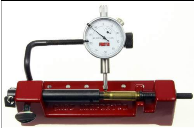
Figure 6. Co-Ax Case and Cartridge Inspector Ready to Measure Neck Wall Thickness
