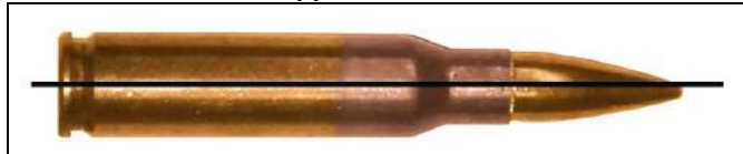
Figure 4. An M80 Ball Round with TIR Off-center Enough to Be Considered a “Tipped” Bullet
