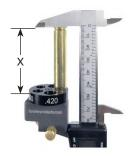
${\sf X}$  = relative measurement between the base of a case to a datum point on its shoulder angle.
