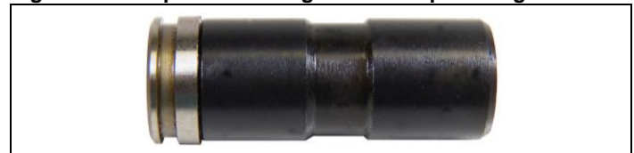
Figure 6. Example Belted Magnum Headspace Gage
