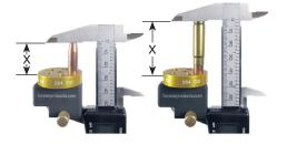
X = relative measurement from the base of a bullet/cartridge to a point on the bullet's ogive, very close to the bullet's major diameter.
