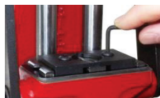
Figure 7. Lower Shell Holder Jaws Change/Adjustment
